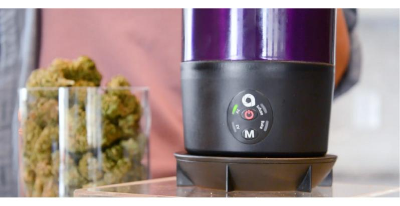
6. After A1 or A2 activation cycles, choose your oil or butter preference and add it to your activated material inside your FX (only up to the Max Fill symbol). Use the M button to toggle to Infuse mode and click the Power button to start the low-temp infusion.
